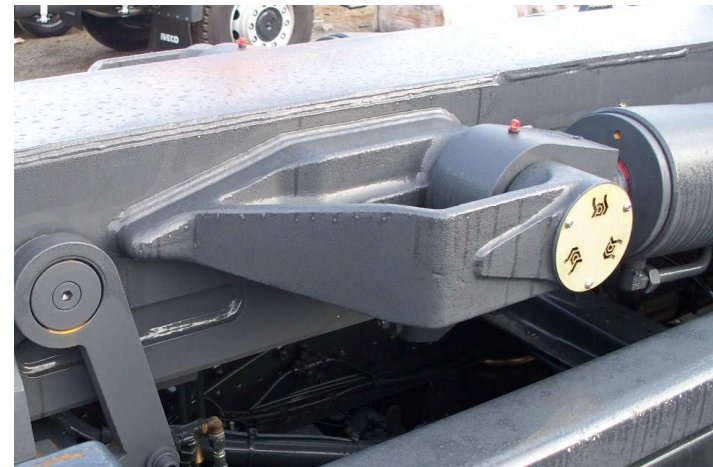
Cylinders fixing to the central body
