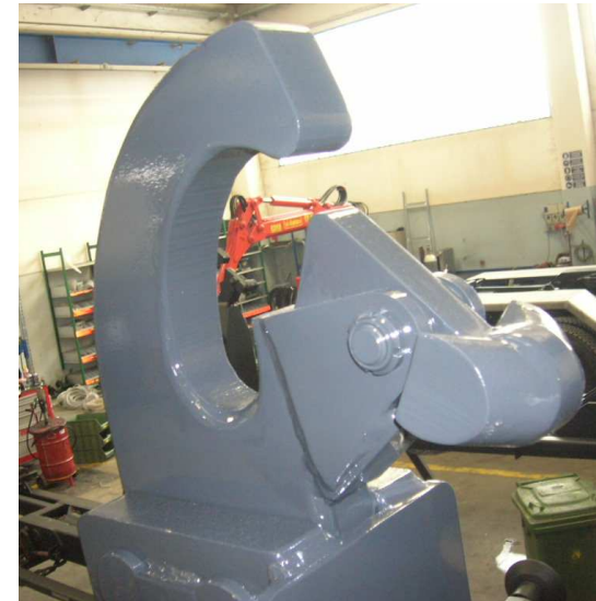
Bolted hook 1460 mm with mechanical security
