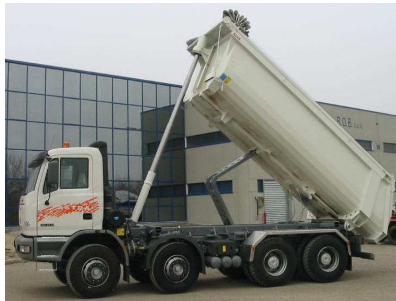
"COMBI" Interchangeable Equipment to use one chassis to do different kinds of work
