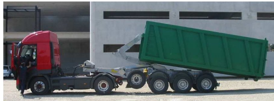
STK 30/7-9 Semi-trailer with built-in hooklift for transport big volumes and containers from 7 to 9 m length
