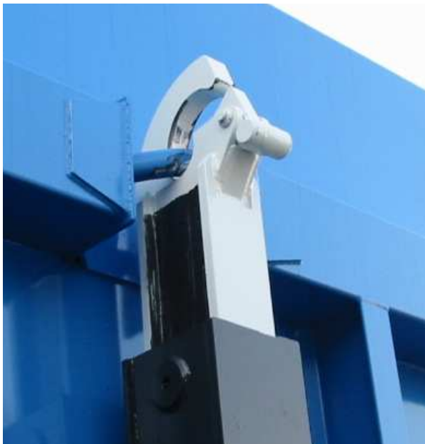
Hook with hydraulic adjustable level 1460/1570 mm
